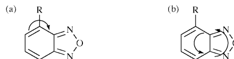
Fig. 2 Structural changes of 4-monosubstituted benzofurazan compounds investigated in this study; (a) twisting of the substituent group, (b) wagging of the benzofurazan skeleton.
